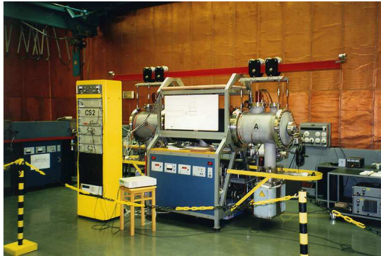
Cesium Clock CS2 of PTB Braunschweig, origin of DCF77 signal
